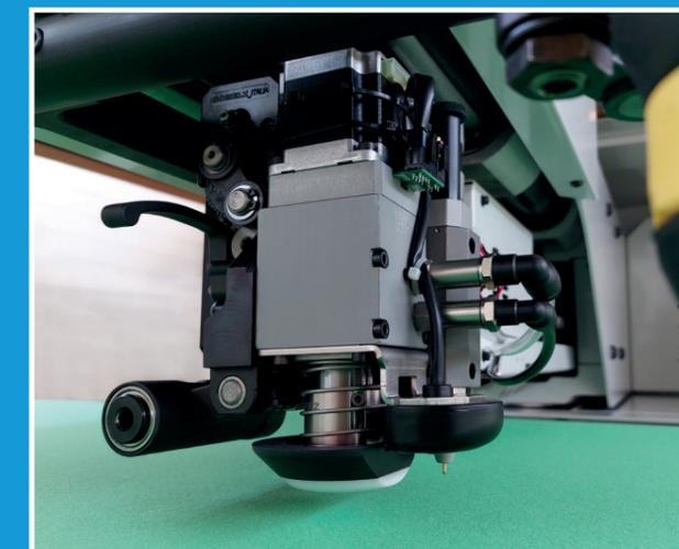
The combination of laser projection, highly visible in all light conditions, and the **telescopic head that keeps the cutting area free** when positioning, offers the best human/machine interaction experience.
