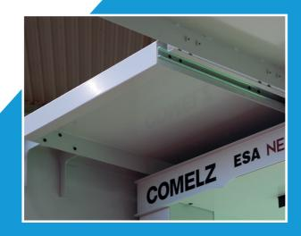
**ADJUSTABLE LIGHT SHIELD** 3 independent sliding panels to isolate the working surface from annoing lights.
